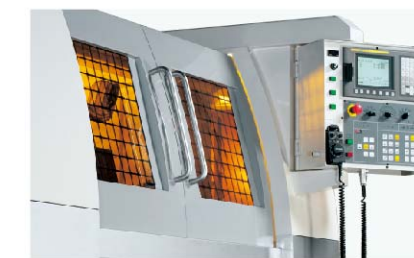
15. Fully Enclosed Splash Guard
