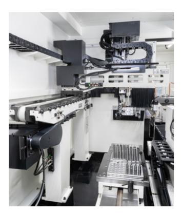
A 3-axes automatic loading/unloading system is offered as a part of the standard machine and it allows unattended and high-speed production. During production, it can carry up to 2 loading trays at the same time with a capacity of up to 1'300 tools
