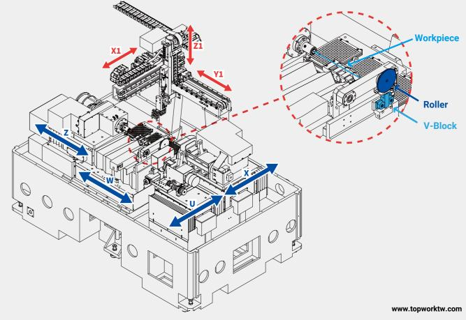
PRECISION CYLINDRICAL PINCH/PEEL GRINDER www.topworktw.co
